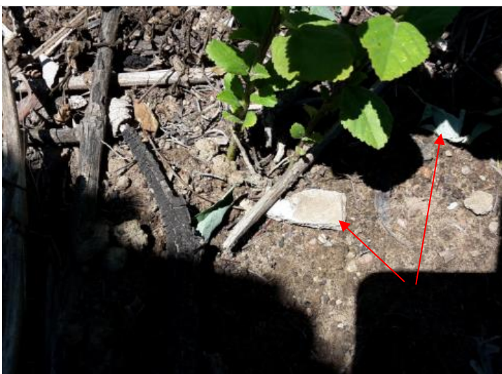
Photograph 12: Example of observed fibre cement fragments on surface of site (see Figure 2).
